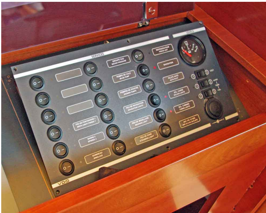
This panel could only open this far due to the wire service loop being too short.
